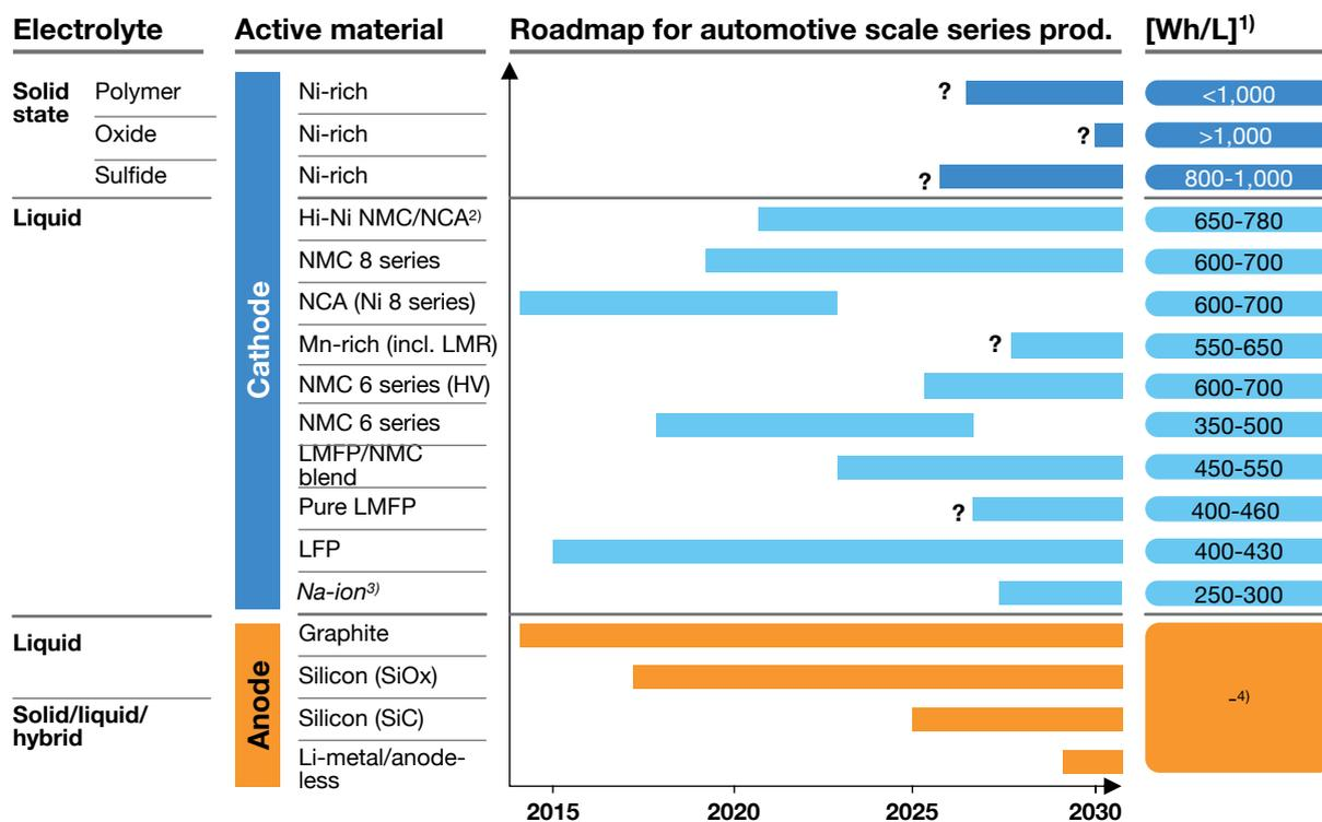
1) Target values for supplier of pouch or prismatic cell; 2) Ni 9 series; 3) Not only cathode chemistry per se but listed for simplification; 4) Primarily driven by cathode chemistry
