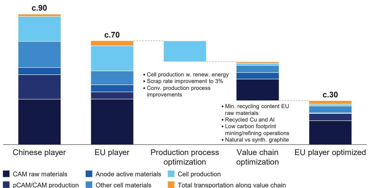
**Figure 1:** Carbon footprint comparison and optimization [kg CO<sub>2</sub>-eq/kWh];
