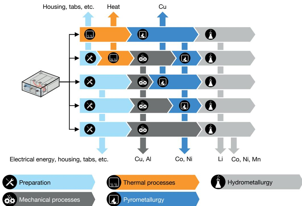
**Figure 28:** Recovered materials in the different recycling stages;
