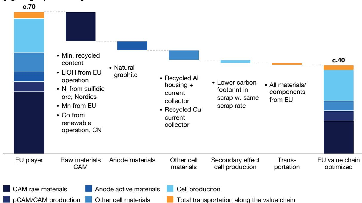
**Figure 7:** Carbon footprint optimization for value chain levers;
