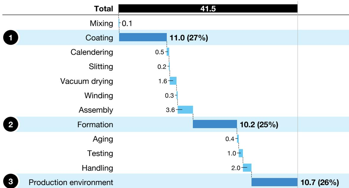
**Figure 11: Energy consumption in battery production; Source: PEM of RWTH Aachen University Production Model**
